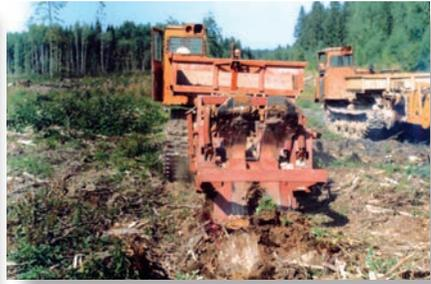
*Left: Making 20–25 cm high layers and plowed furrows for removing excess water with a PSh-1 plow (photo A. Zhigunov).*
