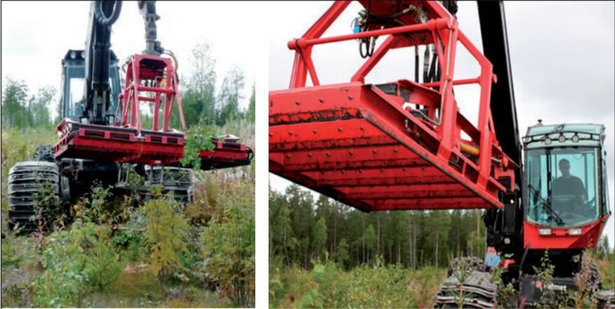
*An uprooting machine in the work (photo T. Saksa)
