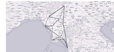
Figure 2. Solutions for the TSP on the Burma14 dataset by the two heuristic approaches, dotted line: VQE ( n_q = 4 , tour length 3499 km), solid line: QA ( n_q = 8 , 3795 km)
