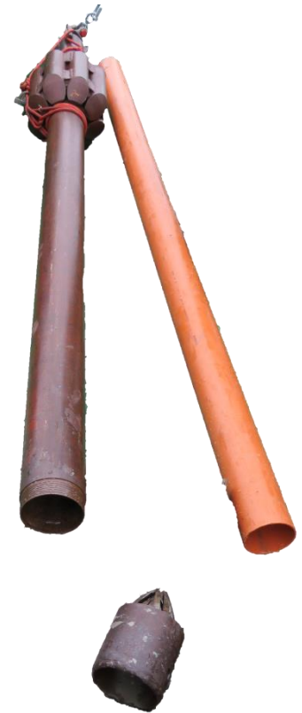
Gravity corer 127 mm in diameter, 3 m long
